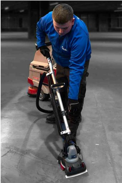
8. Plug suction fitting into tank
