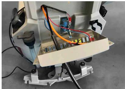
Find the cable and water pipe entry point into the battery compartment. Rear casing or handle assemblies often have entry points you can also drill through switch plates, as shown, for access.
