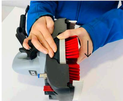
4. Lift machine out of lower mount
